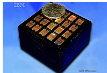
Demonstration of a flip chip mounted 100G transceiver with four wavelength multiplexing at 25 G each.
