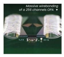
Self aligned µlenses array on PIC
