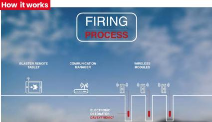
▲ Reliable and secure process for detonator activation thanks to wireless modules that can be controlled from a distance using a tablet interface
