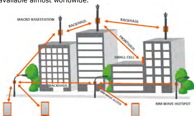
Figure 1: mmW access and backhaul physical architecture.
